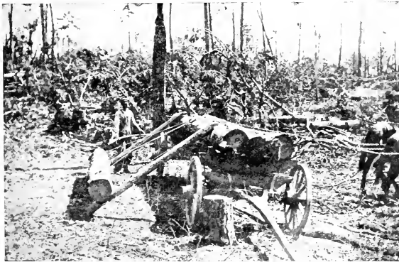
Fig. 57. — Loading a Log Wagon by means of the Crosshaul. The teamster is doing his own loading. Missouri.
